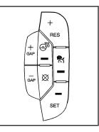
The FCA control is located on the steering wheel.
